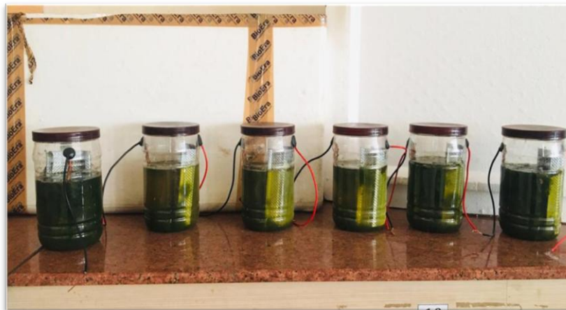
Fig No.3. Microbial Fuel Cells Bottles Connected in series with Algal Water
